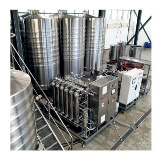
All of our STARS® units are pairable with our crossflow for tartaric stabilization (except the SMART machines) can be combined with our crossflow filtration process. We size your stabilization-filtration unit to meet your production needs.
